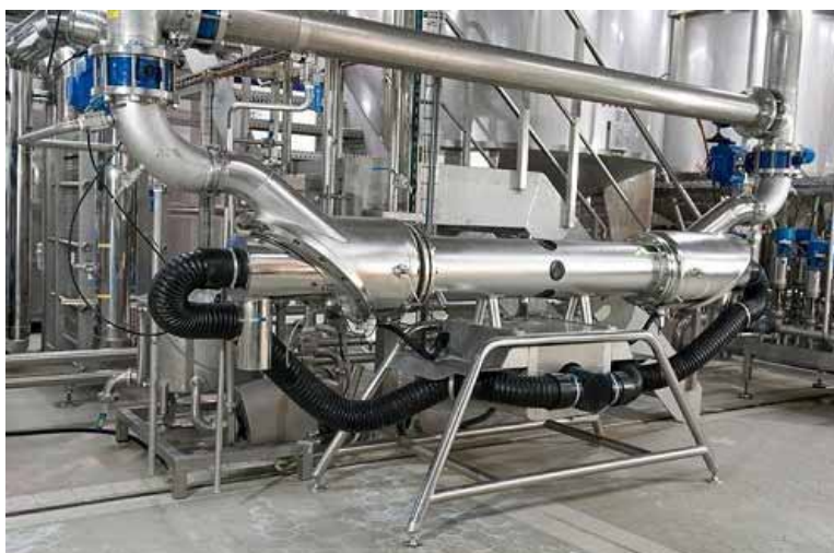
Atlantium's PR-20 at a large dairy plant operating as a non-thermal pasteuriser, having replaced a conventional heat pasteuriser
